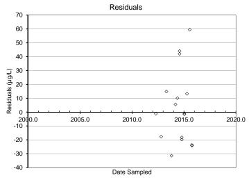
FOD 100% Slope -0.19 p-value 0.02 Slope is negative Regression is acceptable Slope used to estimate degradation rate
