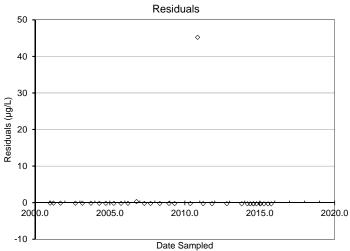
FOD= 9% Slope not calculated p-value not calculated Regression not calculated due to low FOD (< 50%)
