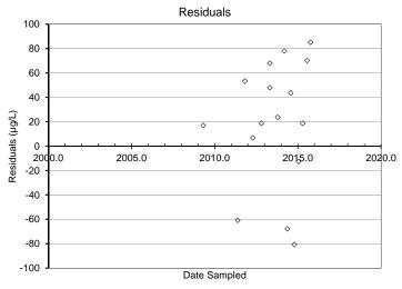
FOD 100% Slope -0.27 p-value 0.041 Regression residuals are appropriately distributed Slope is negative Regression fit is acceptable Slope used to estimate degradation rate
