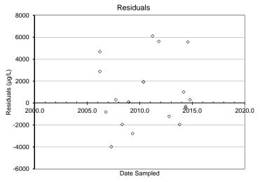
FOD 100% Slope -0.20 p-value <0.01 Slope is negative Regression residuals are biased Slope not used to estimate degradation rate
