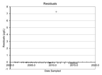
FOD 9% Slope not calculated p-value not calculated Regression not calculated due to low FOD (< 50%)
