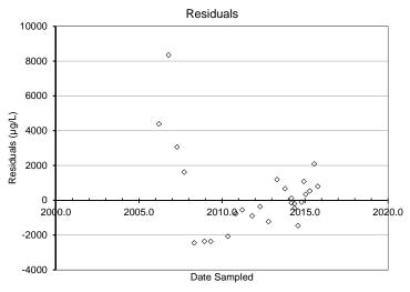
FOD 100% Slope -0.14 p-value < 0.001 Regression residuals are biased Slope is negative Slope not used to estimate degradation rate
