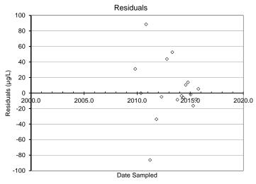
FOD100% Slope 0.015 p-value >0.05 Regression residuals are potentially biased Slope trend is not significant Slope not used to estimate degradation rate
