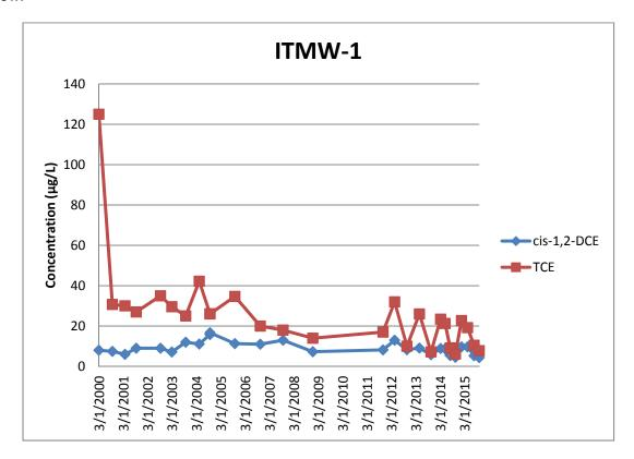
ITMW-17 also had a fairly shallow regression slope (-0.05) for cis-1,2-DCE. A review of the TCE and cis-1,2-DCE data from this location shows that the cis-1,2-DCE is matching the pattern of TCE concentration fairly well as shown in the chart below. Therefore cis-1,2-DCE is not increasing as a result of a MNA stall.
