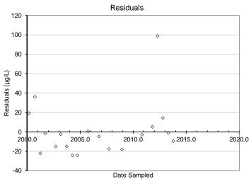
FOD 100% Slope -0.022 p-value >0.05 Regression residuals are appropriately distributed Slope trend is not significant Slope used to estimate degradation rate
