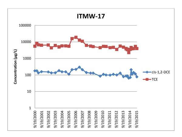
The northern plume degradation rate for VC could not be calculated as only one well (IW-73) contained a sufficient amount of VC data necessary for statistical evaluation via regression analysis. However, the concentration of VC at IW-73 as of October 2015 was 0.59  $\mu$ g/L (J flagged), therefore VC is not being generated at this location in sufficient quantities to affect remedial action levels.
