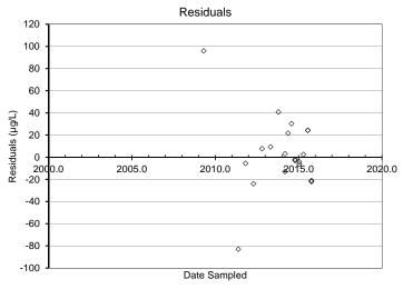
FOD 100% Slope -0.021 p-value 0.521 Regression residuals are appropriately distributed Slope is not significant Slope used to estimate degradation rate
