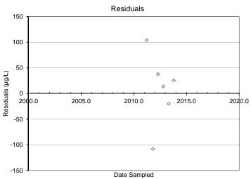
FOD 100% Slope -0.049 p-value >0.05 Residuals are appropriated distributed Slope is not significant Slope used to estimate degradation rate
