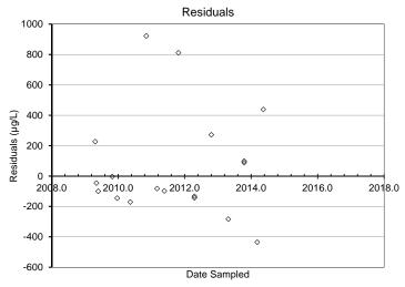
FOD 100% Slope 0.22 p-value <0.01 Regression residuals are potentially biased Slope is not significant Slope not used to estimate degradation rate
