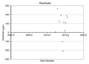
FOD 100% Slope -0.28 p-value >0.05 Regression residuals are appropriately distributed Slope is not significant Slope used to estimate degradation rate
