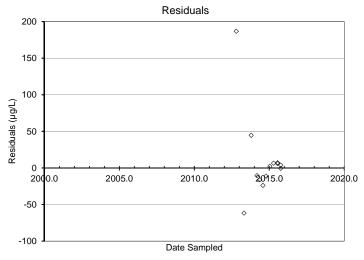
FOD= 100% Slope -0.71 p-value <0.001 Slope is negative Regression residuals are biased Slope not used to estimate degradation rate
