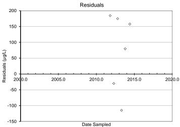
FOD 100% Slope -0.21 p-value >0.05 Regression residuals are potentially biased Slope is trend is not significant Slope not used to estimate degradation rate
